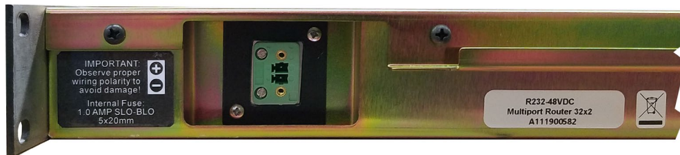
Figure 6: R232-48VDC Pocket Power Supply with removeable terminal receptacle for DC input (shown with mating connector removed)
