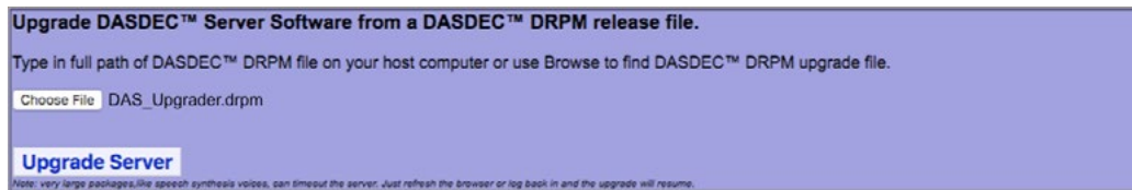
Server Software Upgrade Screen with proper file selected
