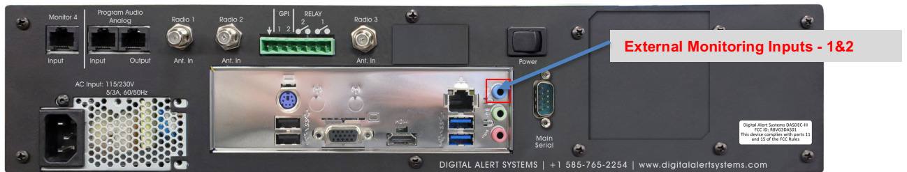
Figure 3. The rear panel of DASDEC-III Model "EL" – dual monitoring inputs only.
