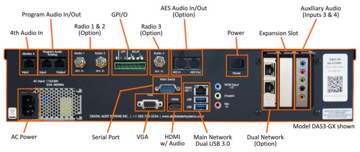
expensive XLRs or difficult to patch terminal strips. The new audio connectors allow simple CAT5/6 wiring with many of the latest audio consoles and devices, following a standard wiring configuration so customers can purchase any number of adaptors (available separately) or craft their own.
